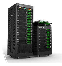
The IT2700 series Multi-channel Modular Power System offers ultra-high power density. The 1U chassis can accommodate up to eight 200W modules or four 500W modules. The modules can be bi-directional DC power supplies, unidirectional DC power supplies, or regenerative DC electronic loads. The modules support mixed configurations, synchronization, and can be connected in series
